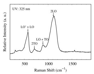
**Fig. 5** The room-temperature backscattering Raman spectra from a 325 nm excitation source.  $LO' + LO~(430-635~cm^{-1})$ , 2TO (720 cm<sup>-1</sup>),  $LO + TO~(850-940~cm^{-1})$  and  $2LO~(1120~cm^{-1})$ .
