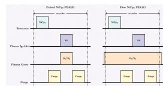
Fig. 1 Schematic of the flow and pulsed PEALD process tested for the deposition of NiO
