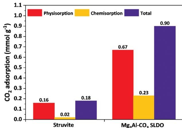
Fig. 4 CO<sub>2</sub> adsorption of struvite and Mg<sub>3</sub>Al-CO<sub>3</sub> SLDO at 40 °C and 100 kPa. The samples were initially calcined at 400 °C for 2 hours.
