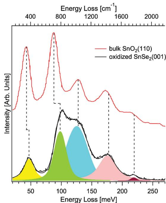
Fig. 4 Vibrational spectra for the oxidized surface of SnSe<sub>2</sub>(001) taken by HREELS. The primary electron beam energy is 4 eV. Experiments were carried out at room temperature. For the sake of comparison, we report also data for bulk SnO<sub>2</sub>(110) (data taken from ref. 155). Reproduced with permission ref. 154.
