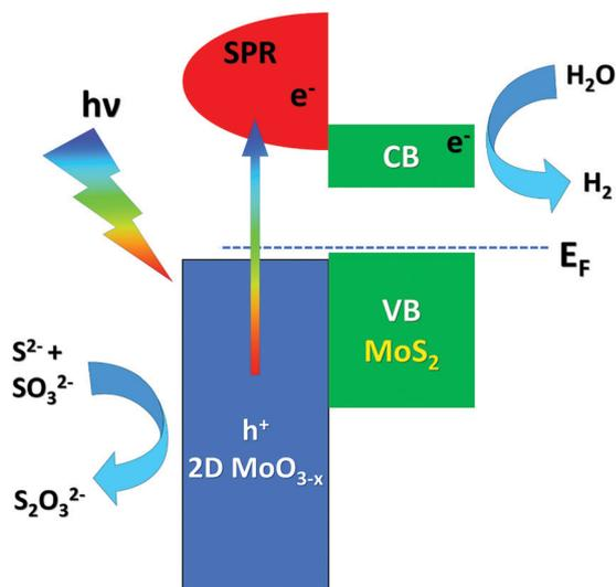
Fig. 3 Energy-level alignment and the mechanism of electron transfer at the MoS<sub>2</sub>/MoO<sub>3</sub> interface. Adapted with permission ref. 141. CB and VB stand for the conduction and valence band, respectively.
