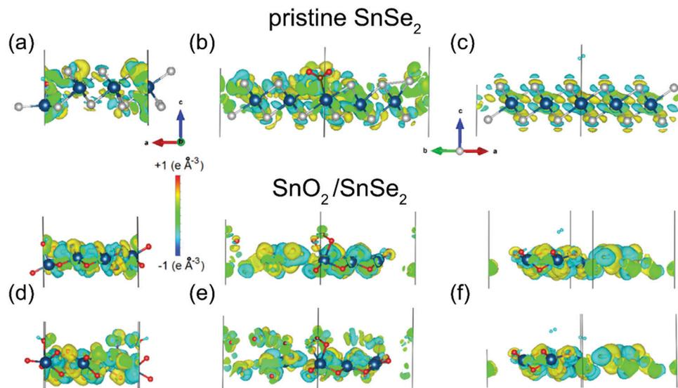
Fig. 5 Changes in the charge densities in (a–c) SnSe<sub>2</sub> or (d–f) SnO<sub>2</sub>/SnSe<sub>2</sub> surfaces after adsorption of (a and d) water, (b and e) nitrogen dioxide and (c and f) hydrogen. For the SnO<sub>2</sub> skin, results for adsorption of a single molecule are shown in the top layer and for the pair of molecules in the bottom layers of the panels. Blue, white and red balls denote Sn, Se, and O atoms, respectively. Reproduced with permission ref. 154.
