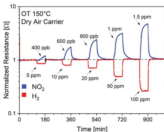
Fig. 6 Dynamic gas responses of the SnO<sub>2</sub>/SnSe<sub>2</sub> heterostructure for gas concentrations of NO<sub>2</sub> (400 ppb–1.5 ppm) and H<sub>2</sub> (5–100 ppm) in a dry air carrier gas at an operational temperature of 150 °C. OT stands for operational temperature. Reproduced with permission ref. 154.
