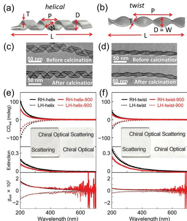
**Fig. 1** 3D illustrations of RH- (a) helical and (b) twisted silica nanoribbons. TEM images of RH- (c) helical and (d) twisted silica nanoribbons.  $CD_{ext}$  (top), extinction (middle), and  $g$ -factor (bottom) spectra of drop-cast films ( $50 \mu\text{g cm}^{-2}$ ) of (e) helical and (f) twisted silica nanoribbons. Inset images show photos of the films of helical and twisted silica ribbons ( $50 \mu\text{g cm}^{-2}$ ) showing the good transparency of the films.
