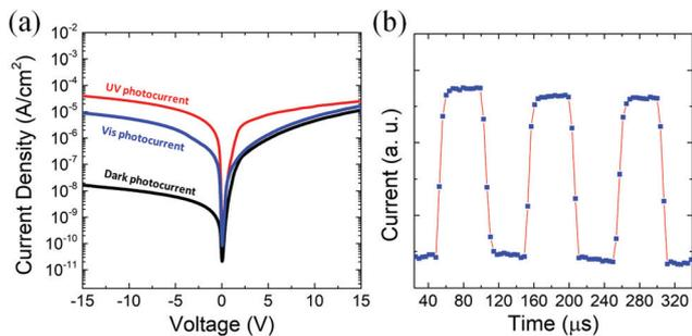
**Fig. 2** (a)  $I$ - $V$  characteristics of the photodetector measured in the dark, under 760 nm visible illumination, and 375 nm UV illumination. (b) Transient response of the heterojunction photodiode with a rising time of 4.3  $\mu$ s and a falling time of 5.2  $\mu$ s measured under ambient conditions.
