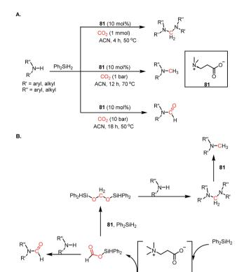
Scheme 35 (A) Hierarchical reductive functionalization of  $CO_2$  with amines using 81. (B) Plausible mechanistic cycle of the hierarchical reductive functionalization of  $CO_2$ .
