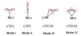
Fig. 2 Common binding modes of the  ${\rm CO_2}$  molecule with metal (considering a single metal).
