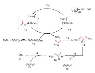
Scheme 4 Converting stoichiometric  $CO_2$  reduction into catalytic process by adding excess  $B(C_6F_5)_3$  and  $Et_3SiH$  to the TMP/ $B(C_6F_5)_3$  system.
