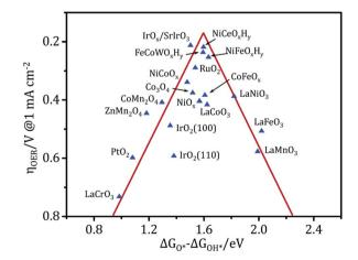
Fig. 7 Activity trends towards the oxygen evolution of (hydro)oxides. The OER overpotential data in the vertical coordinates was measured experimentally and the adsorption energy between two intermediates ( $\Delta G_{\rm O^*} - \Delta G_{\rm OH^*}$ ) in the abscissa is the theoretical data calculated using DFT, where all of the data were obtained from the literature.
