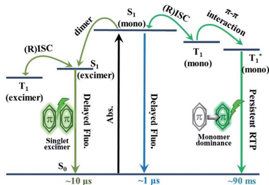
Fig. 6 The proposed PL process of CS-2COOCH<sub>3</sub>.
