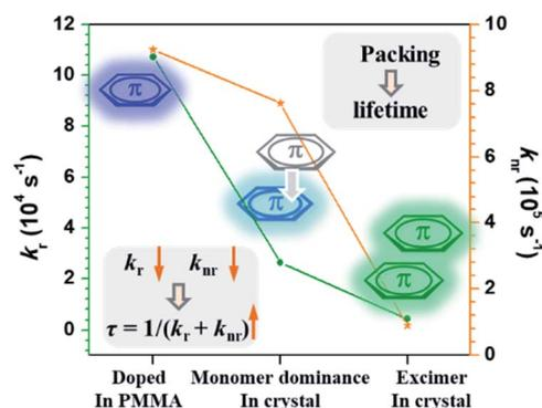
Fig. 5 Changing tendency of the fluorescent radiative rate ( $k_r$ ) and non-radiative rate ( $k_{nr}$ ) for CS-2COOCH<sub>3</sub> in different states.
