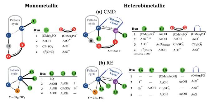
Fig. 2 A generalized representation of (a) concerted metalation—deprotonation (CMD) and (b) reductive elimination (RE) transition states with monometallic and heterobimetallic catalysts.<sup>41</sup> Only the most preferred ligand combinations, obtained by considering a much larger set of possibilities, are shown here. Details of various configurations considered are provided in Section 6 of the ESI.†
