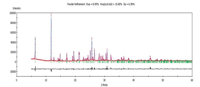
Difference Fig. 1 The Rietveld refinement plot showing an agreement between the calculated and measured X-ray powder diffractograms of the complex.
