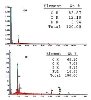
Fig. 3 EDX analysis showing weight% of different elements present in the proposed sensor (a) before and (b) after soaking in 1.0  $\times$   $10^{-3}$  mol L $^{-1}$  Pb(II) ion solution for 1 h at 25 °C.
