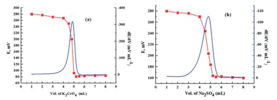
Fig. 7 S-shape and first derivative titration curves for the potentiometric titration of 5.0 mL ( $1.0 \times 10^{-2}$ ) mol L<sup>-1</sup> Pb(NO<sub>3</sub>)<sub>2</sub> solution against (a) 1.0  $\times$  10<sup>-2</sup> mol L<sup>-1</sup> of K<sub>2</sub>CrO<sub>4</sub> and (b) 1.0  $\times$  10<sup>-2</sup> mol L<sup>-1</sup> of Na<sub>2</sub>SO<sub>4</sub>.
