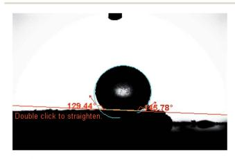
Fig. 6 Contact angle formed by a sessile water drop on a smooth homogenous surface of the used ionophore.
