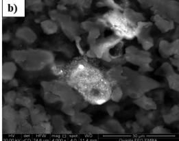
Fig. 2 SEM image of the surface of the proposed sensor (250 mg graphite, 100 mg TCP and 10 mg BMAPP ionophore) (a) before and (b) after soaking in  $1.0 \times 10^{-3}$  mol L<sup>-1</sup> Pb(II) ion for 1 h at 25 °C.
