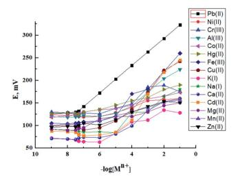
Fig. 1 Potential response of the proposed sensor for different metal ions.
