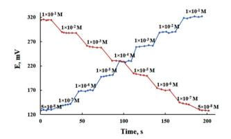
Fig. 5 Dynamic response of the proposed MCPE for step changes of Pb(II) concentration from low-to-high and high-to-low.
