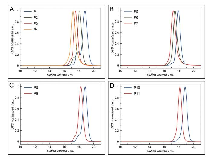
Fig. 1 HFIP GPC elugrams of the synthesised mTz- and TCO-functionalised polymers: (A) mTz-pSar, (B) TCO-pSar, (C) mTz-pGlu(OBn), (D) TCO-pGlu(OBn).
