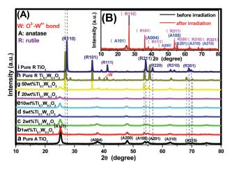
Fig. 1 PXRD patterns of the tested samples: (A) (a) pure anatase  $\text{TiO}_2$ ,  $\text{Ti}_{0.7}\text{W}_{0.3}\text{O}_2/\text{TiO}_2$  NCI of (b) 1 wt%, (c) 2 wt%, (d) 5 wt%, (e) 10 wt%, (f) 20 wt%, (g) 50 wt%, (h) pure rutile  $\text{Ti}_{0.7}\text{W}_{0.3}\text{O}_2$ , (i) pure rutile  $\text{Ti}_{0.7}\text{W}_{0.3}\text{O}_2$ /TiO<sub>2</sub> NCI before and after six cycles of irradiation, respectively.
