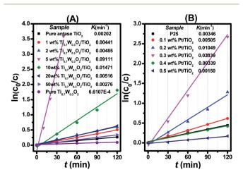
Fig. 7 Dependence of In  $(c_0/c)$  on the irradiation time (t) for: (A) Ti<sub>0.7</sub>W<sub>0.3</sub>O<sub>2</sub>/TiO<sub>2</sub> NCI, (B) P25 and Pt/TiO<sub>2</sub>.
