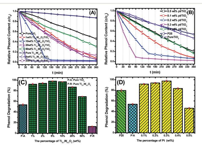
Fig. 6 Photocatalytic degradation of phenol over: (A)  $Ti_{0.7}W_{0.3}O_2/TiO_2$  NCI, (B) P-25 and Pt/TiO<sub>2</sub>, c = concentration,  $c_0 =$  initial concentration. The phenol photocatalytic degradation rates of: (C) Ti<sub>0.7</sub>W<sub>0.3</sub>O<sub>2</sub>/TiO<sub>2</sub> NCI, (D) P-25 and Pt/TiO<sub>2</sub> after 360 min irradiation.
