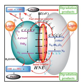
Scheme 1 Proposed phenol photocatalytic degradation mechanism at the Ti<sub>0.7</sub>W<sub>0.3</sub>O<sub>2</sub>/TiO<sub>2</sub> NCI.
