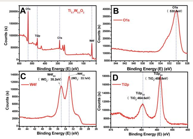
Fig. 4 XPS survey scan spectra of: (A) rutile Ti<sub>0.7</sub>W<sub>0.3</sub>O<sub>2</sub>, and XPS narrow scans of: (B) O 1s, (C) W 4f and (D) Ti 2p of the rutile Ti<sub>0.7</sub>W<sub>0.3</sub>O<sub>2</sub>.
