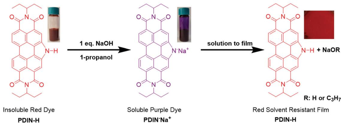
Fig. 1 Chemical structure of PDIN-H. Treatment of a 10 mg mL<sup>-1</sup> slurry of PDIN-H in 1-propanol with 1 molar equivalent of NaOH produces a purple ionic solution. Spin-coating this solution onto a PET substrate yields a red colored organic film owing to the spontaneous protonation of the PDIN<sup>-</sup> anion. This process mimics that of classic acid dyeing of textiles.
