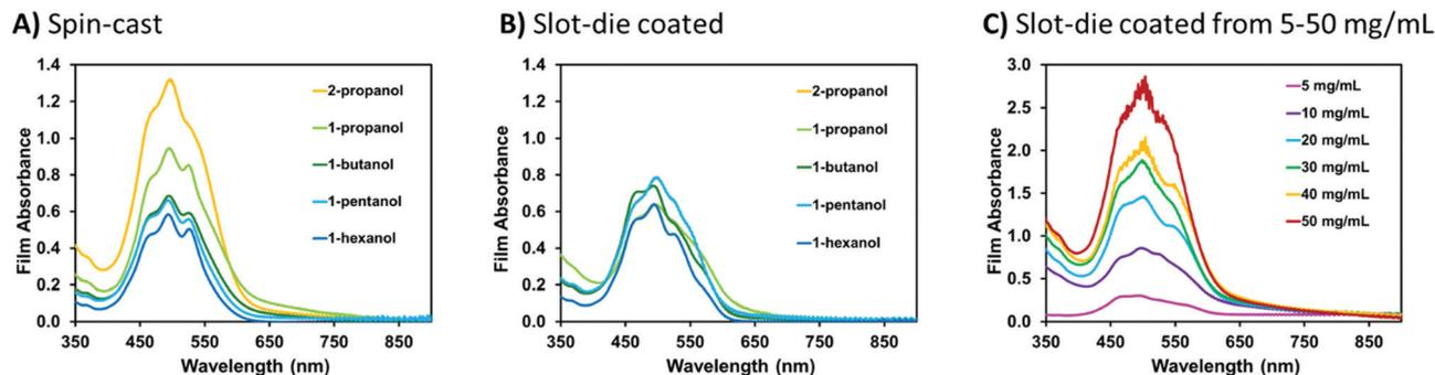
Fig. 5 Optical absorption spectra of (A) PDIN-H films spin-coated from different alcohols at  $10 \text{ mg mL}^{-1}$ , (B) PDIN-H films slot-die coated from different alcohols at  $10 \text{ mg mL}^{-1}$ , and (C) PDIN-H films slot-die coated from 1-propanol at varying concentrations onto PET. In all cases 1 molar equivalent NaOH was added to each pre-deposition solution.
