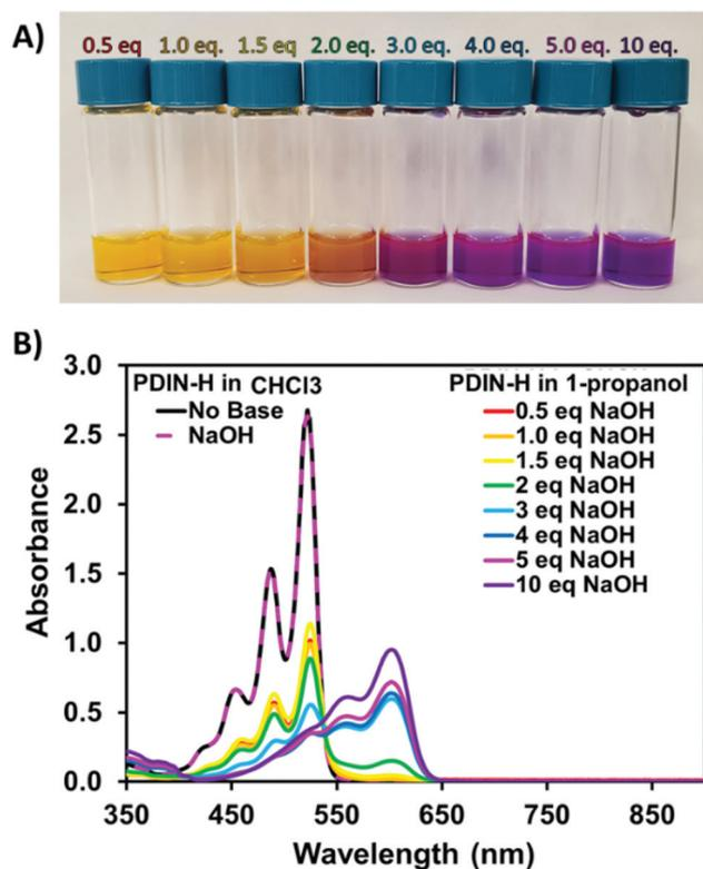
Fig. 2 (A) Image showing the color changes of PDIN-H in 1-propanol solution with varying equivalents of NaOH added. (B) UV-vis spectra of PDIN-H solutions in CHCl<sub>3</sub> with 1 mol equivalent NaOH, and in 1-propanol with 0–10 mol equivalents of NaOH.
