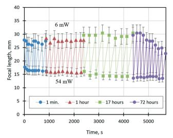
Fig. 9 The dependence of the focal length of the solutocapillary lens (50% mixture of ethylene glycol and ethyl alcohol, 1  $\mu$ l) on the cyclically (10 times for a series) changing power of the laser beam between 6 mW (the upper symbols) and 54 mW (the lower symbols). The time intervals between series when the laser beam is off: 1, 17 and 72 hours. The experiment started in 1 minute after the liquid was deposited in the cell.
