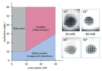
Fig. 10 The stability diagram of the solutocapillary lens (50% mixture of ethylene glycol and ethyl alcohol,  $1 \mu l$ ) operating at different angles of inclination (0-60°) and powers of the laser beam. The borders (dashed lines) between areas in the diagram are drawn approximately. On the right - the images of the test grid for the different tilt angles of the lens and laser beam powers.
