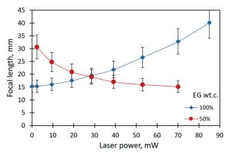
Fig. 4 The focal length of the liquid lenses (1  $\mu$ l in volume) of pure ethylene glycol and its 50% mixture with ethyl alcohol vs. the power of the laser beam.
