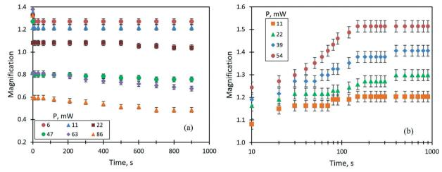
Fig. 8 Evolution of the linear magnification of liquid lenses at different powers of the laser beam: (a) benzyl alcohol (0.6 μl), the thermocapillary mechanism; (b) 50% mixture of ethylene glycol and ethyl alcohol (1 μl), the solutocapillary mechanism.
