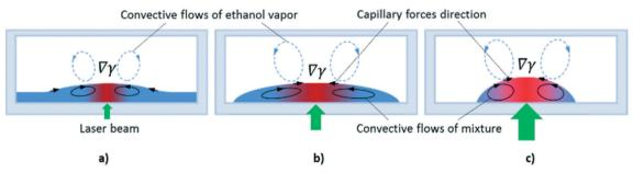
Fig. 3 Schema of the droplet formation process in a layer of liquid mixture induced by the laser beam. ∇y is the concentration surface tension gradient along the interface. (a) The convex deformation of the layer caused by the laser beam; (b) formation of the droplet in the layer; (c) the droplet shrinkage cause by the laser power increasing.
