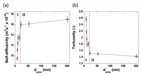
Fig. 7 The pore size dependence of (a) the self-diffusivity of n-octane imbibed within the pores of the alumina carriers and (b) the calculated tortuosity values.
