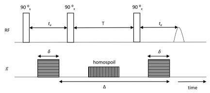
Fig. 1 PGSTE pulse sequence showing gradient pulse duration  $\delta$ , echo time  $t_e$ , storage interval T, homospoil gradient and diffusion time,  $\Delta$ .
