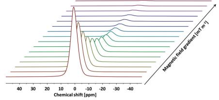
Fig. 5 A typical PFG NMR decay plot of n-octane imbibed within Al<sub>2</sub>O<sub>3</sub> (1) obtained using the PGSTE pulse sequence. Self-diffusion coefficients were obtained by fitting the log attenuations to egn (1). Data collected at atmospheric pressure and 25 °C.
