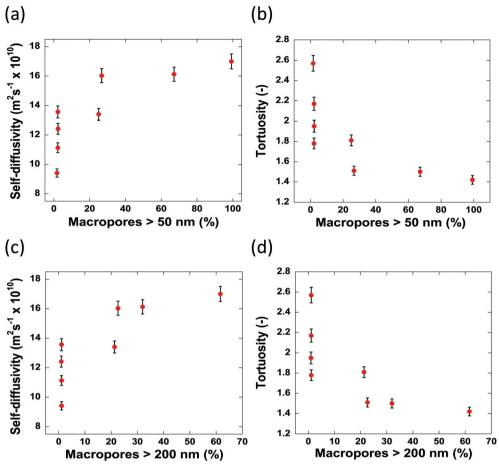
Fig. 8 The effect of the percentage of macropores with a radius greater than 50 nm on (a) the self-diffusivity of n-octane imbibed within the alumina carriers and (b) the calculated tortuosities. Figures (c) and (d) show the effect of the percentage of macropores with a radius greater than 200 nm on the self-diffusivity of imbibed n-octane and the calculated tortuosities, respectively.
