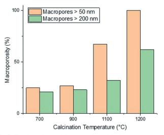
Fig. 3 The dependence of the preparation calcination temperature of the carriers Al<sub>2</sub>O<sub>3</sub> (5)-Al<sub>2</sub>O<sub>3</sub> (8) upon the percentage of macropores with diameter >50 nm and the percentage of macropores with diameter >200 nm within the carrier produced.
