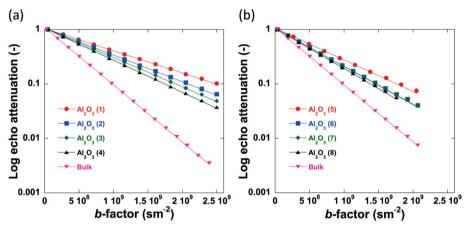
Fig. 6 Log attenuation plots of n-octane imbibed within (a)  $Al_2O_3$  (1)- $Al_2O_3$  (4) and (b)  $Al_2O_3$  (5)- $Al_2O_3$  (8). Solid lines are fitting to eqn (1). Data collected at atmospheric pressure and 25 °C.
