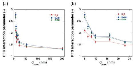
Fig. 9 The pore size dependence of the PFG interaction parameter,  $\xi$ , for water, methanol and ethanol imbibed within (a) the alumina carriers and (b) the alumina carriers with  $Al_2O_3$  (8) omitted to aid comparison of the smaller pore size samples.
