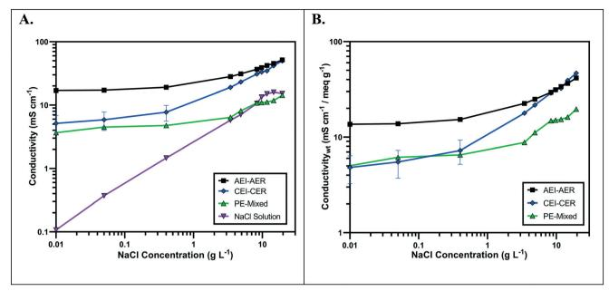
Fig. 3 (A) lonic conductivity of single ion-conducting RWs at various NaCl concentrations. (B) lonic conductivity normalized to ion-exchange capacity at various NaCl concentrations. Error bars in these plots represent the absolute difference (n = 2) from the average for the ionomer RWs.
