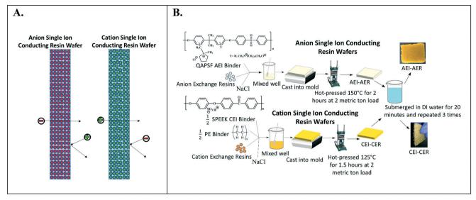
Fig. 2 (A) Illustration of single ion-conducting RWs. (B) Manufacturing scheme for single anion- and single cation-conducting RWs.
