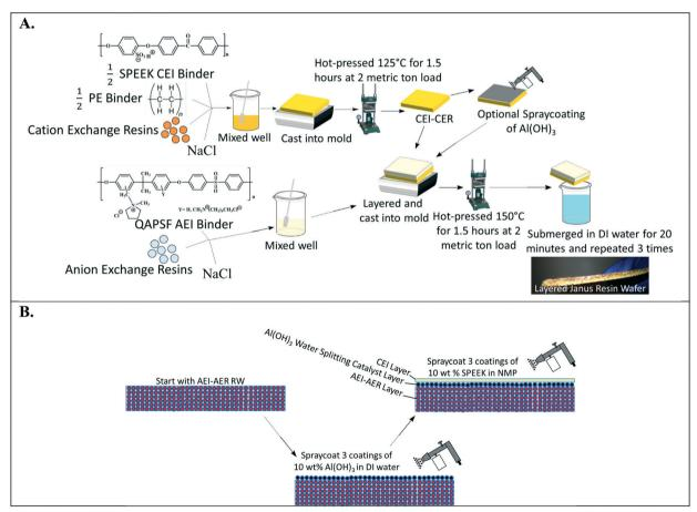
Fig. 5 (A) Manufacturing scheme for symmetric Janus bipolar RW with optional inclusion of a water dissociation catalyst (Al(OH)<sub>3</sub> nanoparticles). (B) Manufacturing scheme for an asymmetric Janus bipolar RW with optional inclusion of a water dissociation catalyst.
