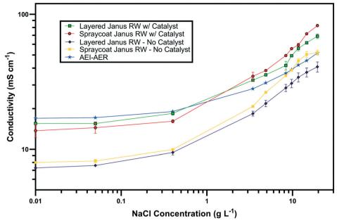
Fig. 7 Ionic conductivity of symmetric and asymmetric Janus bipolar RWs with and without water dissociation catalyst. Error bars represent absolute difference (n = 2) from the average of measurements.
