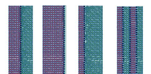
A. Symmetric Janus B. Asymmetric Janus C. Reverse Asymmetric D. Bilayer Janus Bipolar Resin Wafer Bipolar Resin Wafer Janus Bipolar Resin Wafer Bipolar Resin Wafer
