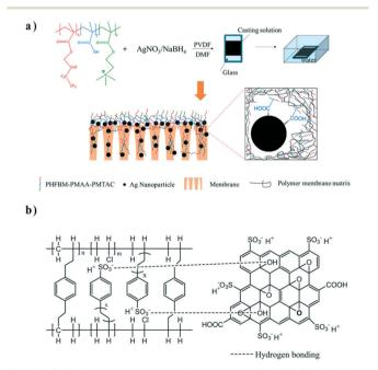
Fig. 4 a) Fabrication process and structure of a PVDF/Ag/PHFBM-PMAA-PMTAC membrane. b) Schematic illustration of the interactions within an interpenetrating network/SGO composite membrane. Reproduced with permission from ref. 52 and 53. Copyright 2019 and 2018, Elsevier.
