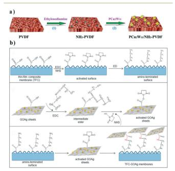
Fig. 5 Fabrication process of a) the PCu<sub>2</sub>W<sub>11</sub>/NH<sub>2</sub>-PVDF interface composite membrane and b) binding GO-Ag nanosheets on the TFC membrane. Reproduced with permission from ref. 66 and 67. Copyright 2017, Elsevier.
