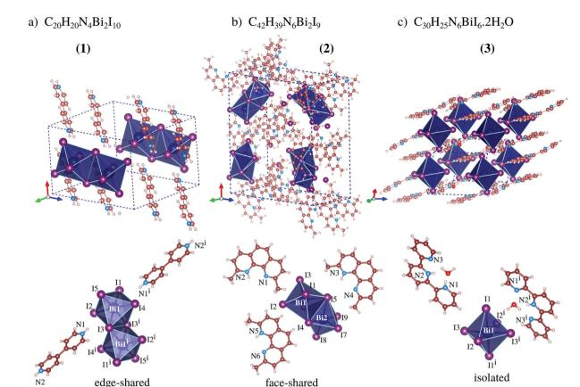
Fig. 1 Experimental crystal structures of perovskites 1, 2 and 3, where the dashed-lines indicate the unit cell, while the octahedra show the frames formed by the Bil<sub>6</sub> ions.
