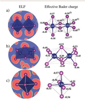
Fig. 4 Electron localization function (ELF) and effective Bader charge (e) of inorganic  $\operatorname{Bi}_{x}\operatorname{I}_{y}^{\delta-}$  moieties of perovskites (a) **1**, (b) **2** and (c) **3**. Along bismuth-iodide planes, the colors blue and red in the ELF plots represent electron charge depletion and accumulation, respectively
