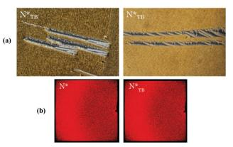
Fig. 5 (a) POM textures seen for the chiral twist-bend nematic phase and (b) X-ray diffraction patterns obtained in the N\* and N\* $_{TB}$  phases for CB6OS:(S)-(2-Me)4OBA.
