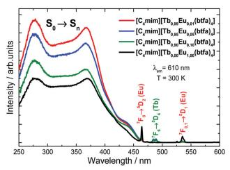
Fig. 3 Excitation spectra for the  $[C_4 \text{mim}][Tb_{1-x}Eu_x(btfa)_4]$  (x = 0.01, 0.05, 0.10 and 1.00) complexes recorded at room temperature (300 K) monitoring the Eu<sup>3+ 5</sup>D<sub>0</sub>  $\rightarrow$  <sup>7</sup>F<sub>2</sub> emission (610 nm).
