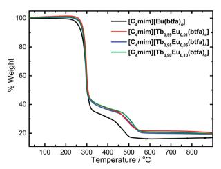
Fig. 1 TGA curves of the  $[C_4 \text{mim}][Tb_{1-x}\text{Eu}_x(\text{btfa})_4]$  ( $x=0.01,\ 0.05,\ 0.10,\ 1.00$ ) complexes recorded under a synthetic air atmosphere at 10 °C min $^{-1}$ .
