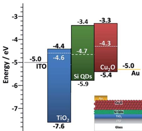
Fig. 6 Non-equilibrated band diagram for the PV device based on Si QDs as active layers,  $\text{Cu}_2\text{O}$  QDs as an electron blocking layer, a  $\text{TiO}_2$  film hole blocking layer and corresponding contacts. Inset: diagram of the layer structure of the device.
