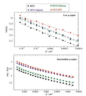
Fig. 2 Guinier plots for HNT/chitosan, HNT/alginate, HNT/HPC and HNT dispersions in D<sub>2</sub>O within the low (0.007 nm<sup>-1</sup>  $\leq q \leq$  0.009 nm<sup>-1</sup>) and the intermediate (0.015  $\text{nm}^{-1} \le q \le 0.02 \text{ nm}^{-1}$ ) regions. The low q Guinier plot is ln(I(q)) vs.  $q^2$  (top), while the intermediate q Guinier plot is  $ln(q \cdot I(q))$ vs.  $q^2$  (bottom). Dashed lines represent the fitting according to eqn (1) and (3).
