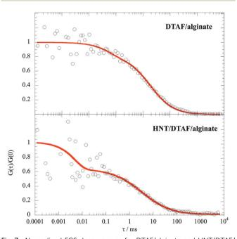
Fig. 7 Normalized FCS decay curves for DTAF/alginate and HNT/DTAF/ alginate mixtures in water. The concentration of DTAF/alginate was set at 0.1 mg dm<sup>-3</sup>, while the overall concentration of alginate was fixed at  $10~{\rm g}~{\rm dm}^{-3}$ . Accordingly, the labelled alginate/HNT mass ratio was  $10^{-4}$  and the mass ratio between the overall alginate and HNT was 0.1. Red lines represent the fitting according to the triplet state model.<sup>56</sup>
