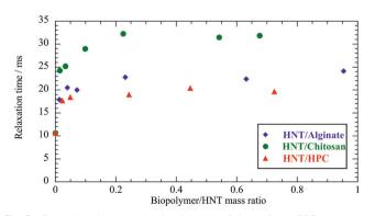
Fig. 5 Relaxation time determined by the fitting of the EBR data as a function of the biopolymer/HNT mass ratio at a HNT concentration of  $0.15 \text{ g dm}^{-3}$  (SANS and FCS experiments were done at 0.1).
