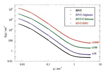
Fig. 1 SANS intensity as a function of q, the magnitude of the scattering vector, for HNT/chitosan, HNT/alginate, HNT/HPC and HNT dispersions in D<sub>2</sub>O. The HNT concentration and the HNT/biopolymer mass ratio were  $80~{\rm g}~{\rm dm}^{-3}$  and 10, respectively.
