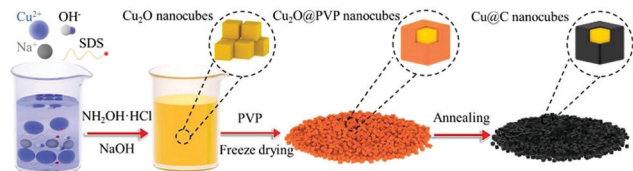
Fig. 13 Schematic diagram of well-aligned Cu@C core-shell nanocube synthesis. Reproduced from ref. 158 with permission from Elsevier B.V., copyright 2019.
