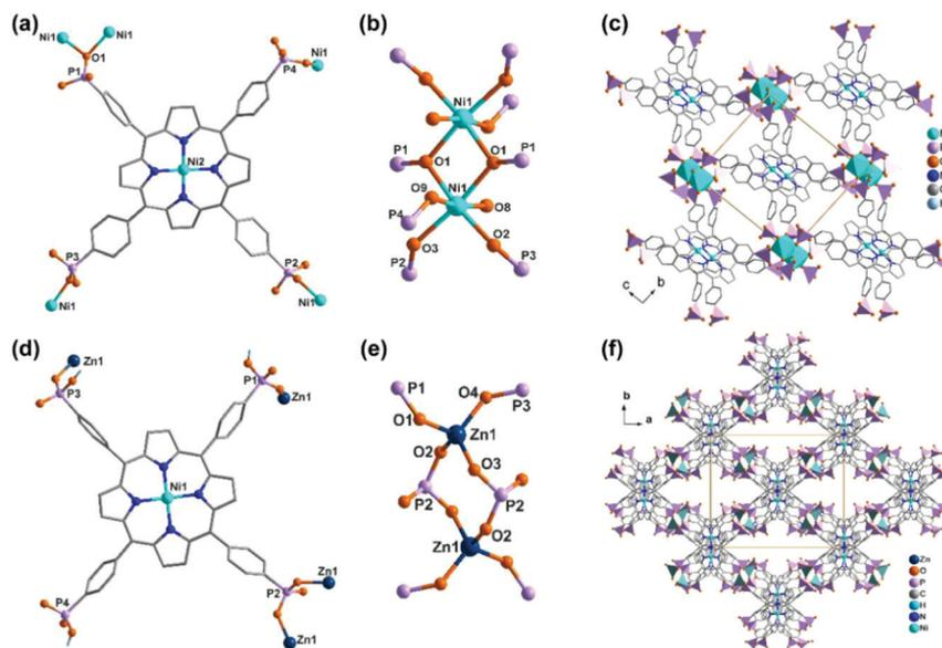
Fig. 10 (a–c) The structure of compound **51**: (a) coordination mode of Ni–H<sub>6</sub>TPPP<sup>2–</sup>, (b) dimeric building unit, (c) packing diagram. (d–f) The structure of compound **53**: (d) coordination mode of Ni–H<sub>6</sub>TPPP<sup>2–</sup>, (e) dimeric building unit, (f) packing diagram. Adapted from ref. 60 and 61.
