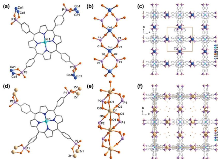
**Fig. 11** (a–c) The structure of compound **54**: (a) coordination mode of Ni-H<sub>4</sub>TPPP<sup>2-</sup>, (b) dimeric building unit, (c) packing diagram. (d–f) The structure of compound **55**: (d) coordination mode of Ni-H<sub>6</sub>TPPP<sup>2-</sup>, (e) dimeric building unit, (f) packing diagram. Adapted from ref. 62 and 63.
