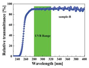
Fig. 2 Relative transmittance through a p-AlGaN UV-B LED (sample-B).
