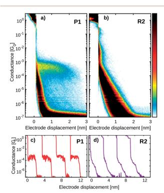
Fig. 4 Two-dimensional conductance vs. displacement histograms built from 10 000 consecutive breaking traces of (a) P1 and (b) R2; no data selection was made. Both measurements were performed with a bias of 100 mV at room temperature. Examples of individual conductance breaking traces for (c) P1 and (d) R2 (with a horizontal offset of 3 nm for clarity).
