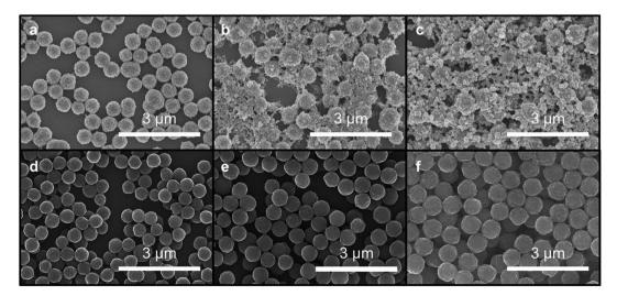
Fig. 4 SEM images of colloidal suspension at 50 equiv.  $h^{-1}$  (a–c) and 1 equiv.  $h^{-1}$  (d–f) of monomer addition. Aliquots were drop-casted after (a, d) 2 equivalents, (b, e) 4 equivalents, and (c, f) 6 equivalents of monomers were added.
