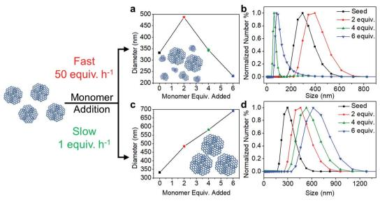
Fig. 3 Trend in the average size of particles with monomer addition at a fast rate of 50 equiv.  $h^{-1}$  and at a slow rate of 1 equiv.  $h^{-1}$ . (a, c) Average size of particles with additional equivalents of monomers (b, d) corresponding number percent distribution.
