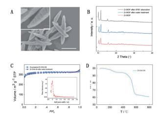
Fig. 2 Scanning electron microscopy images of prepared Zr-CAU-24 crystals with different magnification times. Scale bar: 1  $\mu m$  ((A), inset). PXRD of Zr-CAU-24 crystals before and after water treatment and AFB1 absorption, (B) and  $N_2$  adsorption/desorption isotherms (C) of Zr-CAU-24 crystals before and after 24 h water treatment. TGA result of as-prepared Zr-CAU-24 crystals (D).
