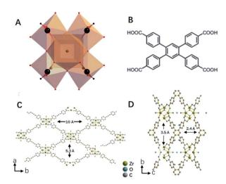
Fig. 1 Crystal structure of Zr-CAU-24 that is constructed from the  $[Zr_6(\mu_3-O)_4(\mu_3-OH)_4]^{12+}$  clusters (A) and TCPB<sup>4+</sup> molecules (B). Ballstick models of Zr-CAU-24 crystals (C) and (D).
