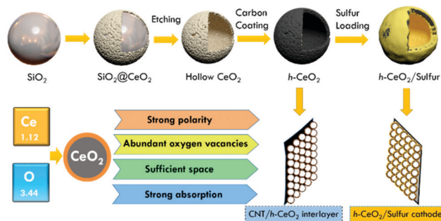
Fig. 1 Illustration of synthetic procedures of a h-CeO 2 /sulfur cathode and a CNT/h-CeO 2 interlayer for Li-S batteries.
