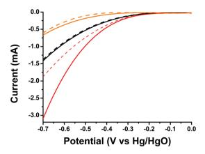
Fig. 5 LSV curves of oligothiophene 1 (orange), SG (black) and 1/SG (red), recorded under light illumination (solid) and dark (dashed) conditions, in the  $O_2$  saturated aqueous 0.1 M KOH electrolyte.
