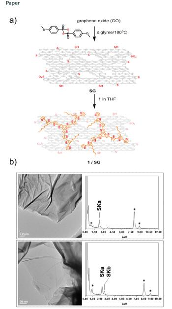
Fig. 1 (a) Preparation of the 1/SG ensemble featuring oligothiophene 1 immobilized onto S-doped graphene via  $\pi-\pi$  interactions. (b) Representative HR-TEM images and EDX analysis of SG (upper panel) and 1/SG (lower panel). With asterisks are marked EDX signals from the copper mesh grid.
