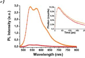
Fig. 2 (a) Full Raman spectra ( $\lambda_{\rm exc}$  633 nm) and (b) expansion of the G-band of 1/SG (red), GO (grey), SG (black) and 1/GO (blue). (c) Photoluminescence spectra ( $\lambda_{\rm exc}$  441 nm) of 1 (orange) and 1/SG (red) obtained in benzonitrile. Inset: Photoluminescence lifetime decay graphs.
