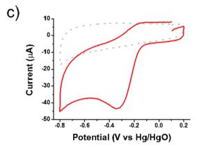
Fig. 3 Cyclic voltammographs of (a) SG, (b) 1 and (c) 1/SG in nitrogen (dotted) and oxygen (solid) saturated aqueous 0.1 M KOH electrolytes.
