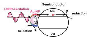
Fig. 1 Hot electron transfer mechanism.
