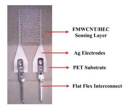
Fig. 5 Photograph of the printed sensor.
