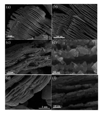
Fig. 3 SEM images of (a and b)  ${\rm Ti_3C_2}$ , (c and d) TF, and (e and f) TOH samples.
