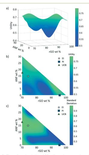
Fig. 6 Three-dimensional plot of (a) utility and contour plots of (b) utility and (c) standard deviation vs. composition. Circular points represent the initial experimental data while the star, square, and triangle represent recommendations from the model based on either expected improvement (EI), probability of improvement (PI), or upper confidence bound (UCB), respectively.
