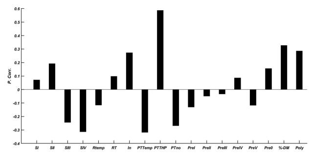
Fig. 1 Relative Pearson correlation coefficients (P. corr. maximum range: –1 to +1) for the conditioning processes related to the obtained CEC concentrations. Statistical data related to available information on biogas processing and CEC concentrations measured in the respective digestate samples. % DM and PTTHP showed positive and significant correlations (P.corr. = 0.57 and 0.59 respectively, p < 0.05).
