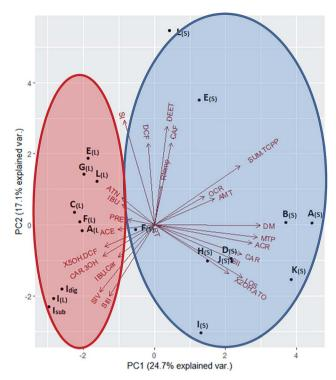
Fig. 3 Bi-plot for Principal Component Analysis (PCA) conducted for variables potentially influencing the CEC distribution profile in the analysed digestate samples. Red circle (liquid digestates); blue circle (solid digestates). All abbreviations are explained in Table S1† and Fig. 1.
