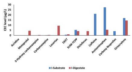
Fig. 4 Concentration comparison between the target CECs in a substrate (blue  $-l_{\text{sub}}$ ) and a digestate sample (red  $-l_{\text{dig}}$ ) collected from an experimental reactor at station I. Please note these samples originate from the same production plant but are not produced during the same biogas process.
