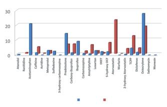
Fig. 2 Average relative distributions of selected CECs (100% = sum CECs) detected and quantified in solid (red) and liquid (blue) digestate samples.
