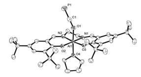
Fig. 3 Molecular structure of 2a-THF in the crystal<sup>25</sup> (ellipsoids are shown at 50% probability; hydrogen atoms and three toluene molecules are omitted for clarity). Selected bond distances [A] and angles [°]: C1-P1 1.587(5), C1-O1 1.228(5), Al1-O1 1.920(3), Al1-O2 1.802(3), Al1-O3 1.796(2), Al1-O4 2.040(3), C1-O1-Al1 137.5(2), O1-C1-P1 178.5(3).
