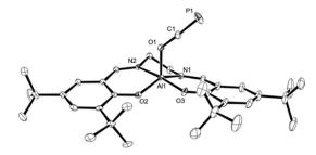
Fig. 1 Molecular structure of 2a in the crystal<sup>25</sup> (ellipsoids are shown at 50% probability; hydrogen atoms are omitted for clarity). Selected bond distances [A] and angles [°]: C1-P1 1.5646(9), O1-C1 1.2538(10), Al1-O1 1.8206(7), Al1-O2 1.7670(6), Al1-O3 1.7901(6), C1-O1-Al1 131.38(6), O1-C1-P1 177.61(8).
