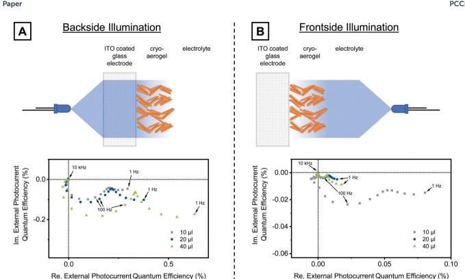
Fig. 5 IMPS responses of cryoaerogel coated photoelectrodes with different film thicknesses. For the preparation of all samples, a 28 mM NPL solution dispersed in  $1 \times 10^{-2}$  M KOH was applied. The samples were irradiated either from the backside (A) or from the frontside (B). The sketches (top) illustrate the differences between both types of irradiation. All IMPS spectra (bottom) were measured at a bias potential of 300 mV.
