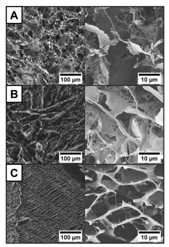
Fig. 3 SEM images of different CdSe NPL cryoaerogel coatings. The concentration of Cd2+ in the original aqueous NPL solutions increases from panel A to C (A: 10 mM, B: 28 mM, and C: 70 mM). For the preparation of each sample, 20  $\mu$ L of the respective NPL solution was used. The KOH concentration was kept constant at  $1 \times 10^{-2}$  M.
