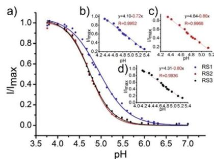
**Fig. 11** (a) Sigmoidal fitting of the maximum emission fluorescence intensity at 590 nm for probes **8**, **9** and **10**. Inset: (b) The linearity of probe **8** in the pH range of 4.34–5.35. (c) The linearity of probe **9** in the pH range of 4.34–5.13. (d) The linearity of probe **10** in the pH range of 4.16–5.25. Copyright 2015 Elsevier.
