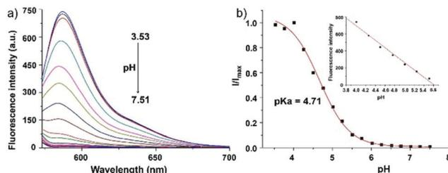
Fig. 5 (a) Fluorescence spectra of probe **3** (10  $\mu$ M) in buffer at various pH values; (b) fluorescence spectra at 584 nm with pH values according to the fluorescent pH titration (pH 3.53–7.51),  $\lambda_{\text{ex}}$  = 563 nm. The inset shows the linear relationship of fluorescence intensity at 584 nm and pH values from 4.0 to 5.5 ( $R = 0.98101$ ). Copyright 2013 Elsevier.
