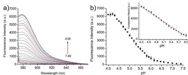
Fig. 57 (a) Fluorescence spectra of probe **38** (1  $\mu\text{M}$ ) in buffers at different pH values; (b) fluorescence intensity at 583 nm with pH values according to the fluorescence pH titration (pH 4.00–7.40),  $\lambda_{\text{ex}} = 563 \text{ nm}$ . The inset shows the linear relationship of fluorescence intensity at 583 nm and pH values from 4.20 to 6.00 ( $R = 0.99523$ ). Copyright 2015 Royal Society of Chemistry.
