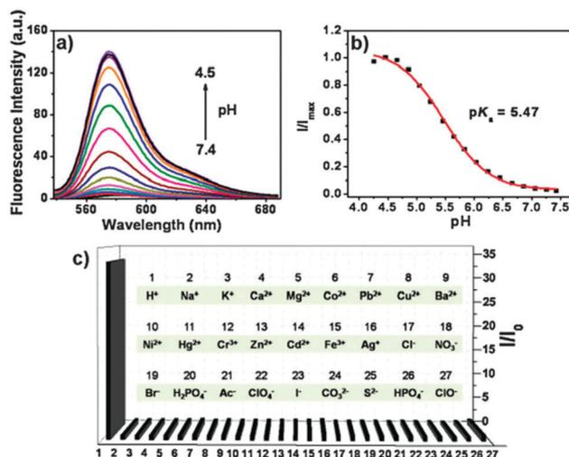
Fig. 17 (a) Fluorescence spectra of probe **13** at various pH values in Britton–Robinson buffer solution,  $\lambda_{\text{ex}} = 525 \text{ nm}$ . (b) pH titration curve of probe **13**,  $\lambda_{\text{ex}} = 559 \text{ nm}$ ,  $\lambda_{\text{em}} = 578 \text{ nm}$ . (c) Fluorescence responses (578 nm) of probe **13** to miscellaneous ions in water:  $50 \mu\text{M}$  for  $\text{H}^+$ ,  $200 \mu\text{M}$  for the other ions. Copyright 2012 Royal Society of Chemistry.
