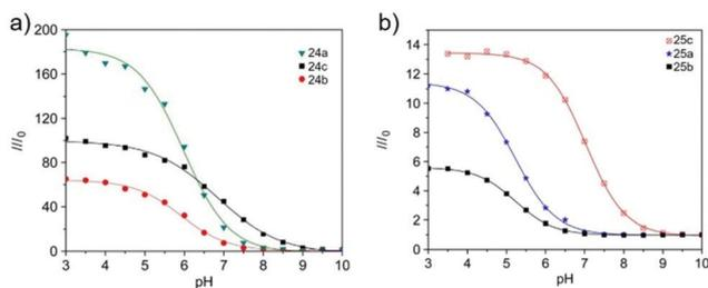
**Fig. 36** (a) Fluorescence intensity (at 517 nm) ratios of probes **24a–c** from pH 3 to pH 10.  $I_0$  is the fluorescence intensity at pH 10. Excitation wavelength for emission spectra was 405 nm. Concentrations of the sensors were  $5 \mu\text{M}$ . (b) Fluorescence intensity (at 517 nm) ratios of thin films **25a–c** from pH 3 to pH 10.  $I_0$  is the fluorescence intensity at pH 10. Excitation wavelength for emission spectra was 405 nm. Copyright 2010 Elsevier.
