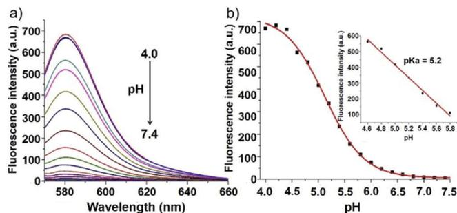
Fig. 15 (a) Change in the fluorescence spectra of probe **12** ( $1 \mu\text{M}$ ) in aqueous solution containing DMSO (B–R buffer : DMSO = 95 : 5, v/v) with decreasing pH from 7.4 to 4.0 ( $\lambda_{\text{ex}} = 560 \text{ nm}$ ). (b) Sigmoidal fitting of the pH-dependent fluorescence intensity at 580 nm. Inset: The good linearity in the pH range of 4.6–5.8. Copyright 2015 Elsevier.
