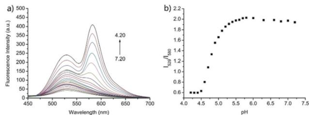
**Fig. 23** (a) Fluorescence spectra of probe **18** (5  $\mu$ M) in the B-R buffer/EtOH (9/1, v/v) solution at different pH values (7.20, 7.00, 6.80, 6.60, 6.30, 6.00, 5.80, 5.70, 5.60, 5.50, 5.40, 5.30, 5.20, 5.10, 5.00, 4.90, 4.80, 4.70, 4.60, 4.50, 4.40, 4.30, and 4.20); and (b) the plot of the emission ratios of  $R$  at  $I_{529}/I_{580}$  versus pH values;  $\lambda_{\text{ex}} = 390$  nm. Copyright 2015 Royal Society of Chemistry.
