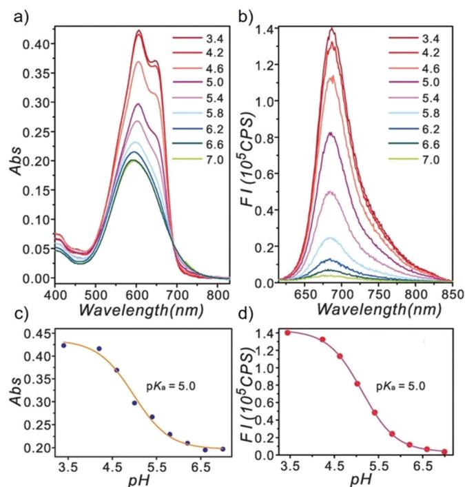
Fig. 38 Optical responses of probe **26a** towards various pH values with disodium hydrogen phosphate–citric acid buffers containing 1% DMSO. (a) Absorption spectra; (b) emission spectra ( $\lambda_{\text{ex}} = 600 \text{ nm}$ ); (c) absorption changes with different pH values monitored at 607 nm; (d) fluorescence intensity changes with different pH values monitored at 686 nm. Copyright 2013 Royal Society of Chemistry.
