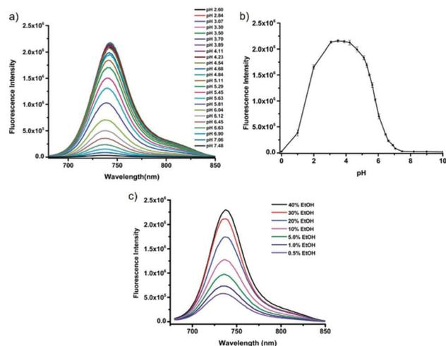
**Fig. 48** Fluorescent spectra of 5  $\mu\text{M}$  fluorescent probe **31** at different pH values in 40 mM citrate–phosphate buffer solution containing 40% ethanol (a) and pH effect on fluorescence intensity of fluorescent probe **31** at 743 nm with three repeated measurements (b). Fluorescence spectra of 5  $\mu\text{M}$  fluorescent probe **34** in 40 mM citrate–phosphate buffer solution at pH 4 containing different concentrations of ethanol (c). Copyright 2014 Royal Society of Chemistry.
