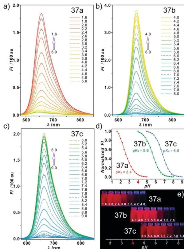
Fig. 56 pH activable emission properties of probes **37a–c** (10  $\mu\text{M}$ ,  $\lambda_{\text{ex}}$  = 570 nm) in disodium hydrogen phosphate–citric acid buffers containing 10% DMSO: (a) probe **37a**; (b) probe **37b**; (c) probe **37c**; (d) normalized fluorescence intensities of probes **37a–c** at different pH values at (a) 657 nm, (b) 668 nm, and (c) 663 nm; (e) photograph of pH-dependent red emissions under a 365 nm lamp in a darkroom. Copyright 2015 American Chemical Society.
