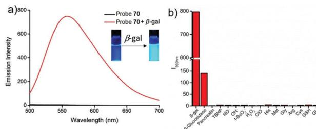
**Fig. 118** (a) The emission of probe **70** with or without  $\beta$ -gal ( $\lambda_{\text{ex}} = 460$  nm). Inset: Images irradiated with 365 nm ultraviolet light. (b) Fluorescence intensity of **70** (10  $\mu\text{M}$ ) in response to the test species in a PBS buffer solution at 560 nm excited at 460 nm. Copyright 2017 Elsevier.
