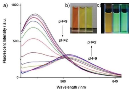
Fig. 50 (a) Fluorescence spectra ( $\lambda_{\text{ex}} = 480 \text{ nm}$ ) of probe **35** ( $2 \mu\text{M}$ ) at different pH values; (b) the color change of probe **35** ( $1 \text{ mM}$ ) in  $20 \text{ mM}$  PBS buffer at different pH values under the condition of visible light; (c) the color change of probe **35** ( $1 \text{ mM}$ ) in  $20 \text{ mM}$  PBS buffer at different pH values under UV light irradiation. Copyright 2014 Elsevier.
