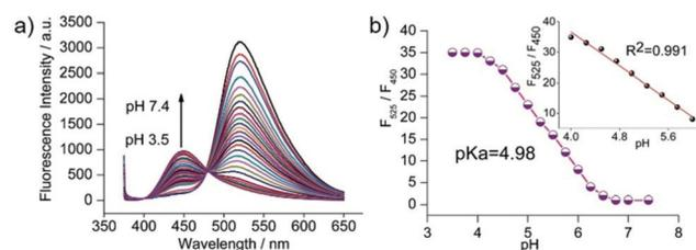
**Fig. 13** (a) Fluorescence emission spectra of probe **11** (1  $\mu$ M) in PBS buffer (10 mM) at different pH values. (b) Plot of  $F_{525}/F_{450}$  (the ratio of the fluorescence intensity of probe **11** at  $\lambda_{em} = 525$  nm and  $\lambda_{em} = 450$  nm) versus pH. Inset: The linear relationship between  $F_{525}/F_{450}$  and pH in the pH range of 4.0–6.3. Copyright 2015 Royal Society of Chemistry.
