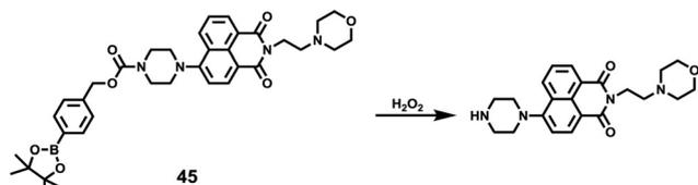
**Scheme 34** Fluorescent probe **45** for  $\text{H}_2\text{O}_2$ .
