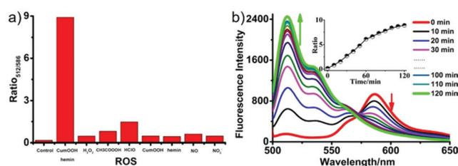
Fig. 82 (a) Fluorescence ratio (512/586) change of probe **54** towards different ROS. (b) Changes of fluorescence wavelength of probe **54** in pH  $\sim 5$  PBS (containing 30% methanol) in the presence of 1  $\mu\text{M}$  hemin and 1 mM CumOOH, excited at 488 nm. Copyright 2015 American Chemical Society.
