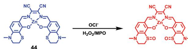
Scheme 33 Fluorescent probe **44** for  $H_2O_2$ .
