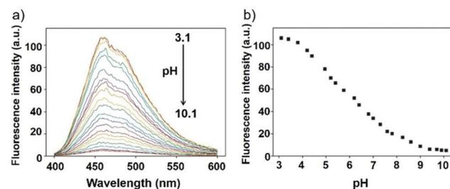
Fig. 34 (a) The fluorescence change of probe **23** in Britton–Robinson buffer at different pH values; (b) the fluorescence intensity at 460 nm depending on different pH values,  $\lambda_{\text{ex}} = 360 \text{ nm}$ . Copyright 2013 Royal Society of Chemistry.
