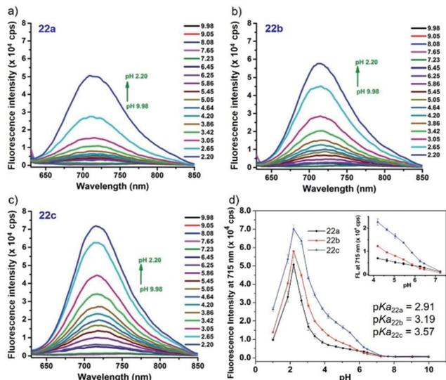
Fig. 31 (a–c) Emission spectra of fluorescent probes **22a–c** (5  $\mu\text{M}$ ) in buffer solution at different pH values. (d) Fluorescent responses of probes **22a–c** to different pH values in buffer solutions. Inset: Zoomed fluorescence intensity responses of probes **22a–c** to pH in the window between cytoplasm pH and lysosomal pH. Copyright 2015 Royal Society of Chemistry.
