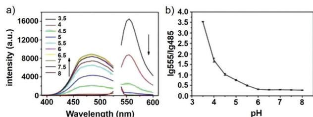
Fig. 19 pH dependent ratiometric fluorescence emission of probe **15**. (a) Fluorescence emission spectra of probe **15** (10  $\mu\text{g mL}^{-1}$ ) at pH 3.5–8.0 under dual-wavelength excitation ( $\lambda_{\text{exc}}$  at 300 nm for dansyl group, 532 nm for R6G-lactam). (b) pH titration curves of lg ratios between fluorescence emission of R6G-amide ( $I_{555\text{nm}}$ ) and that of dansyl group ( $I_{485\text{nm}}$ ). Copyright 2013 Elsevier.
