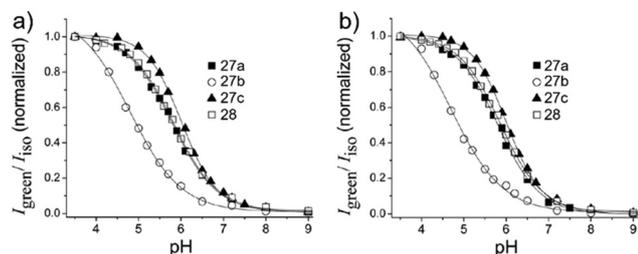
Fig. 41 (a) Plots of  $I_{\text{green}}/I_{\text{iso}}$  versus pH for probes **27a–c** and **28** determined in one-photon mode. The excitation wavelength is 360 nm. (b) Plots of  $I_{\text{green}}/I_{\text{iso}}$  versus pH for probe **27a–c** and **28** determined in two photon mode. Data in (b) are normalized at the maximum  $I_{\text{green}}/I_{\text{iso}}$ . The excitation wavelength for two-photon mode is 740 nm. Copyright 2013 American Chemical Society.
