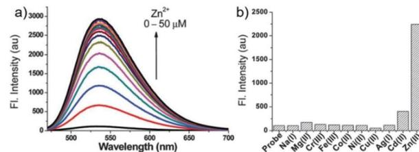
Fig. 112 (a) Fluorescence titration of probe **67** (10  $\mu\text{M}$ ) with  $\text{Zn}(\text{ClO}_4)_2$  in a pH 5.0 MES buffer containing 1% EtOH. (b) Fluorescence intensity changes of probe **67** (10  $\mu\text{M}$ ) with various metal ions (10  $\mu\text{M}$ ) in 1% EtOH containing a pH 5.0 MES buffer. All the fluorescence data were obtained under excitation at 450 nm. Copyright 2016 Royal Society of Chemistry.
