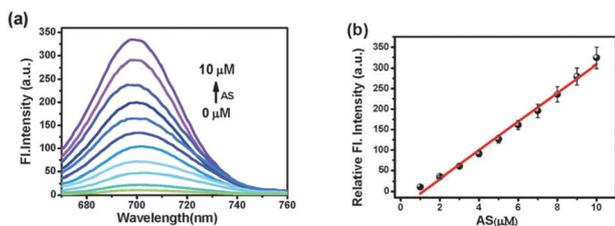
Fig. 107 (a) Fluorescence responses of **65** ( $2 \mu\text{M}$ ) to different concentrations of Angel's salt (AS) with emission ranging from 670 to 760 nm.  $\lambda_{\text{ex}} = 690 \text{ nm}$ . (b) Relationship between the relative fluorescence intensity at 700 nm and concentrations of AS (0, 1, 2, 3, 4, 5, 6, 7, 8, 9, 10  $\mu\text{M}$ ). Fluorescence spectra were acquired in HEPES buffer solution (10 mM, 0.5% DMSO, 0.5% TW 80, pH 5.0). Copyright 2014 Royal Society of Chemistry.
