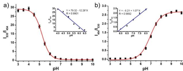
Fig. 61 Fluorescence intensity ratios  $I_{530}/I_{454}$  (a) and  $I_{454}/I_{530}$  (b) of  $5 \mu\text{M}$  **41** in B-F buffers (5% MeOH) at various pH values. Insets are the linear plots of fluorescence intensity ratio to pH;  $\lambda_{\text{ex}} = 380 \text{ nm}$ . Copyright 2016 American Chemical Society.
