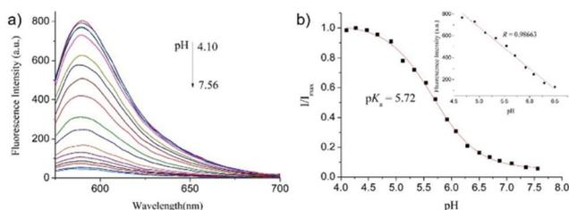
**Fig. 7** (a) Fluorescence spectra of probe **4** (10  $\mu\text{M}$ ) in aqueous solution (Britton–Robinson buffer–EtOH, 9 : 1, v/v) with different pH values; (b) pH titration curve of probe **4**,  $\lambda_{\text{ex}} = 563 \text{ nm}$ ,  $\lambda_{\text{em}} = 589 \text{ nm}$ . The inset shows the linear relationship of fluorescence intensity at 589 nm and varying pH values from 4.6 to 6.5. Copyright 2014 Elsevier.
