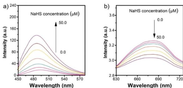
Fig. 93 The changes of fluorescence spectra of **58** in the presence of different concentrations (0.0, 5.0, 10.0, 17.0, 20.0, 40.0, and 50.0 μM) of NaHS in FBS. (a)  $\lambda_{\text{ex}} = 435$  nm; (b)  $\lambda_{\text{ex}} = 510$  nm. Copyright 2017 Royal Society of Chemistry.
