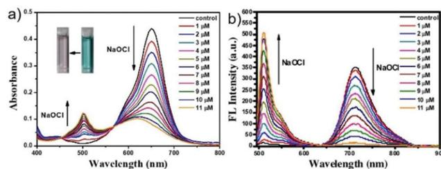
**Fig. 74** (a) UV-vis spectra of probe **51** (5  $\mu\text{M}$ ) upon addition of NaOCl (0–10  $\mu\text{M}$ ) in PBS (10 mM) solution (ethanol/water = 1/1, v/v, pH 7.4). Inset: The color of probe **51** (5  $\mu\text{M}$ ) in the absence and presence of NaOCl (10  $\mu\text{M}$ ). (b) Fluorescence emission of probe **51** (5  $\mu\text{M}$ ) upon the addition of increasing concentrations of NaOCl in PBS (10 mM) solution (ethanol/water = 1/1, v/v, pH 7.4). Copyright 2017 Elsevier.
