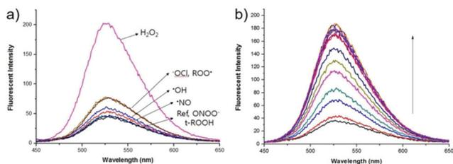
**Fig. 66** (a) Fluorescence spectra of probe **45** (2  $\mu\text{M}$ ) with various ROS (200  $\mu\text{M}$ ) and (b) fluorescence titration of probe **45** (2  $\mu\text{M}$ ) upon addition of  $\text{H}_2\text{O}_2$  (0–100 eq.) in PBS (pH 7.4) solution containing 1% DMF after incubation for 2 h at 25  $^\circ\text{C}$  at an excitation wavelength of 405 nm, and excitation and emission slit widths of 3 and 5 nm, respectively. Copyright 2015 Nature.
