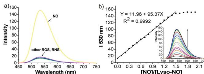
Fig. 102 (a) Selectivity of **63** (11 μM) fluorescence response for NO over other reactive nitrogen and oxygen species (5.0 equiv.) in 20 : 80 CH<sub>3</sub>CN–H<sub>2</sub>O solution at pH 5.0 (in 10 mM phosphate buffer). (b) Intensity at 530 nm vs. NO concentration under the same conditions. Inset: Changes in fluorescence spectra of **63** (11 μM) upon addition of different amounts NO solution (0–2.0 equiv.). Copyright 2012 American Chemical Society.
