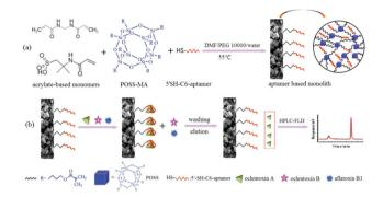
Scheme 1 Schematic of the preparation schemes for the PMAA monolithic column (a) and the diagram of affinity recognition of OTA (b).
