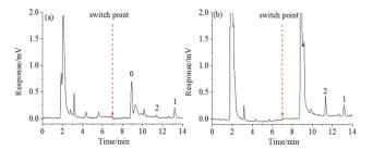
Fig. 6 Nonspecific adsorption of OTB on the PMAA monolith (a) and PEAA monolith (b) peak 0: background compound, peak 1: ochratoxin A, peak 2: ochratoxin B. The concentrations of OTA and OTB were  $0.2 \text{ ng mL}^{-1}$  and  $10 \text{ ng mL}^{-1}$ , respectively.
