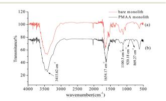
Fig. 2  $\,$  FT-IR spectra of the bare monolith (a) and the PMAA monolith with 5.0% POSS-MA (b).
