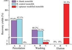
**Fig. 4** Recoveries of OTA with various monoliths in the effluent liquid of different stages. (A) Bare monolith; (B) ssDNA control monolith; (C) PMAA monolith with 5.0% POSS-MA. The concentration of OTA was 10 ng  $\rm mL^{-1}$ .
