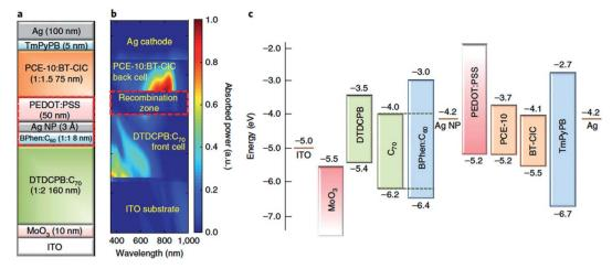
Fig. 11 Tandem device architecture published by Che et al. showing (a) schematic of double junction device; (b) simulated absorbed optical power distribution (relative); (c) energy level diagram. Reprinted by permission from Springer Nature: Che et al., Nat. Energy, Copyright 2018. 100
