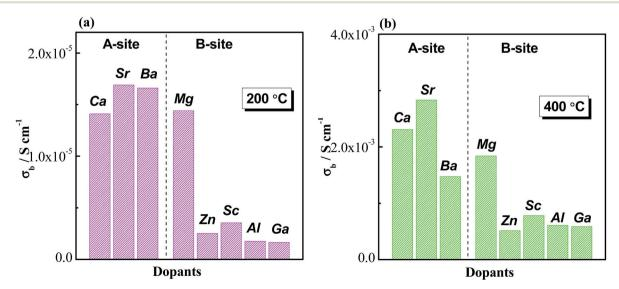
Comparison of bulk conductivity,  $\sigma_{\rm b}$ , with A-site and B-site acceptor-dopants at (a) 200 °C and (b) 400 °C.
