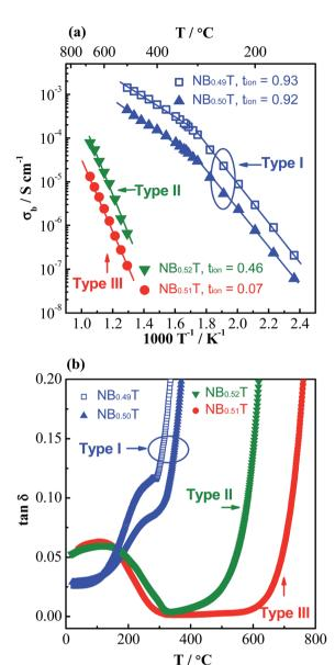
Fig. 1 (a) Arrhenius plot of bulk conductivity,  $\sigma_{\rm b}$  and (b) dielectric loss,  $\tan \delta$ , at 1 MHz *versus* temperature for NBT with various A-site Bi nonstoichiometry:  $Na_{0.5}Bi_{0.49}TiO_{2.985}$ ,  $NB_{0.49}T$ ;  $Na_{0.5}Bi_{0.5}TiO_3$ ,  $NB_{0.50}T$ ;  $Na_{0.5}Bi_{0.51}TiO_{3.015}$ ,  $NB_{0.51}T$ ;  $Na_{0.5}Bi_{0.52}TiO_{3.03}$ ,  $NB_{0.52}T$ . Replotted after ref. 29
