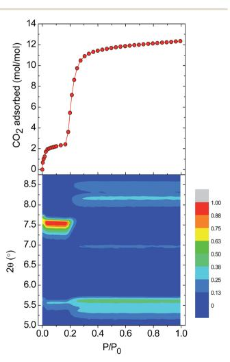
Fig. 4 (top) The adsorption branch of the  $CO_2$  uptake measurements performed at 195 K on 1-a. (bottom) A contour plot of the evolution of the Bragg peaks over the range  $2\theta=5.0-8.75^{\circ}$  as a function of  $P/P_0$ . The intensity of the peaks is relative to the strong peak observed at 7.54° over the pressure range  $P/P_0=0.035-0.18$ .
