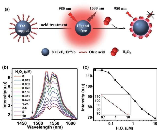
Fig. 3 (a) Process and principle of homogeneous assay of  $\text{H}_2\text{O}_2$  by employing  $\text{NaCeF}_4:\text{Er}/\text{Yb}$  as the probe. (b) NIR-II emission spectra of ligand-free  $\text{NaCeF}_4:\text{Er}/\text{Yb}$  NCs after the addition of different concentrations of  $\text{H}_2\text{O}_2$  upon excitation at 980 nm. (c) Calibration curve for the  $\text{H}_2\text{O}_2$  assay. The inset shows the linear range ( $0.078\text{--}10 \mu\text{M}$ ) of the calibration curve.
