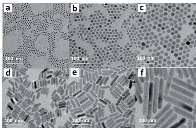
**Fig. 1** NaCeF<sub>4</sub>:Er/Yb NCs synthesized *via* a high-temperature co-precipitation method at 320 °C for (a) 20 min, (b) 25 min, (c) 30 min, (d) 45 min, (e) 60 min and (f) 90 min, respectively. The size of NaCeF<sub>4</sub>:Er/Yb NCs can be estimated by randomly analyzing 200 particles.
