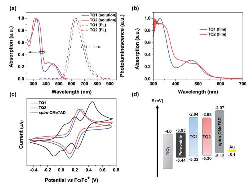
Fig. 2 (a) Absorption and emission spectra of TQ1 and TQ2 in  $CH_2Cl_2$ . (b) Absorption spectra of TQ1 and TQ2 in the thin film state. (c) CV spectra of TQ1, TQ2 and spiro-OMeTAD. (d) Energy-level diagram of perovskite solar cells with different HTMs (energy levels of the perovskite,  $TiO_2$  and Au are taken from ref. 8).
