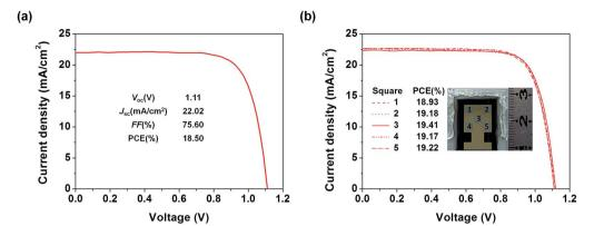
Fig. 7 (a) The J-V curves for the optimized large area (1.02 cm<sup>2</sup>) devices using TQ2 as the HTM. (b) J-V curves measured from five different spots with an aperture area of 0.09 cm<sup>2</sup> selected from the large area device.
