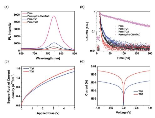
Fig. 5 (a) Steady-state PL spectra of the MAPbl $_3$  perovskite films with or without capping different HTMs. (b) Time resolved photoluminescence decay at 770 nm for the pristine perovskite film and the perovskite films capping different HTMs. (c) The space-charge-limited-current (SCLC) measurements of hole only devices with the configuration of ITO/PEDOT:PSS/HTM/Au. (d) The conductivity measurements of **TQ1** and **TQ2**.
