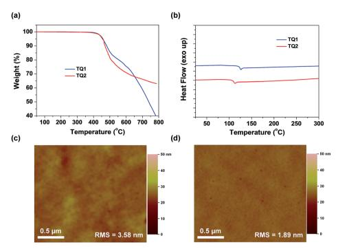
Fig. 3 (a) Thermogravimetric analysis of **TQ1** and **TQ2** measured with a heating rate of  $10\,^{\circ}$ C min $^{-1}$ . (b) The second DSC heating traces of HTMs previously heated and cooled with a scan rate of  $10\,^{\circ}$ C min $^{-1}$  under a nitrogen atmosphere. (c and d) Top-view AFM images of **TQ1** and **TQ2** thin films deposited on the perovskite layer, respectively.
