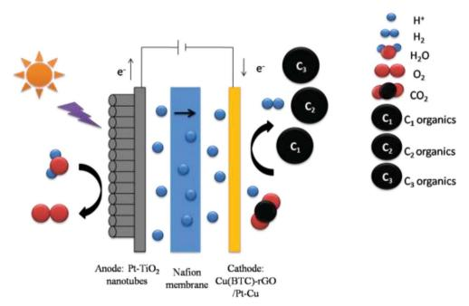
Fig. 1 Schematic of photoelectrochemical cell for CO<sub>2</sub> reduction.
