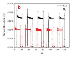
Fig. 6 Electric current densities with different cathodes used: Cu(BTC)-rGO/Pt-Cu foam cathode (a), Cu(BTC)/Pt-Cu foam cathode (b).
