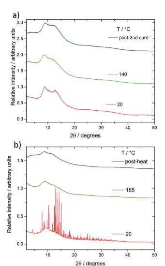
Fig. 5 (a) Stacked pXRD patterns for 70 : 30 wt% sulfur—perillyl alcohol copolymer at room temperature, after heating to 140 °C to 'cure' the detected trace  $\rm S_8$  crystals, and after 24 hours back at room temperature. (b) Stacked pXRD patterns for a slurry of sulfur and perillyl alcohol monomer, after heating to 185 °C to induce reaction, and after 24 hours at room temperature.
