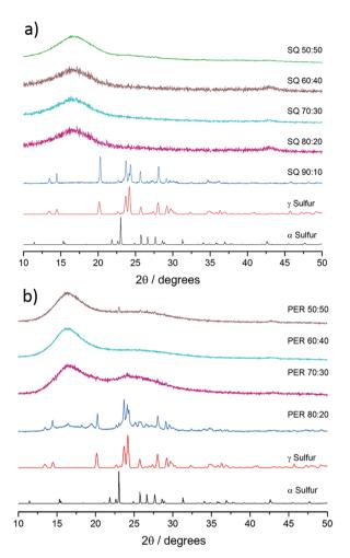
Fig. 3 (a) Stacked p-XRD patterns for different sulfur: squalene copolymer ratios and polymorphs of elemental sulfur and (b) stacked p-XRD patterns for different sulfur: perillyl alcohol copolymer ratios and polymorphs of elemental sulfur.
