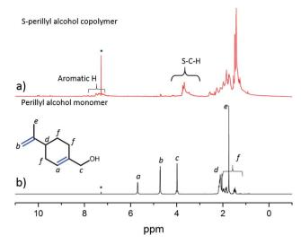
Fig. 2  $\,^{1}$ H NMR for both the sulfur–perillyl alcohol 50: 50 copolymer (a) and the perillyl alcohol monomer (b). Loss of vinylic proton resonances indicate a successful crosslinking by addition across the double bonds, though some aromatic H environments are detected, suggesting some possible hydrogen abstraction. The formation of new peaks in the 3.5–4 ppm region is consistent with the formation of C–S bonds. \*= chloroform.
