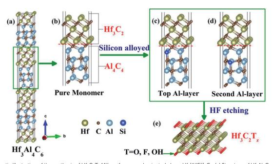
Fig. 2 Schematic illustration of the synthesis of  $Hf_3C_2T_z$  MXene from nanolaminated phase  $Hf_3[Al(Si)]_4C_6$ . (a) Structure of  $Hf_3Al_4C_6$ , (b) structure of pure  $Hf_3Al_4C_6$  monomer, (c) and (d) structure of two  $Hf_3Al_4C_6$  monomers with different silicon alloying, and (e) side view of  $Hf_3C_2$  MXene. Reprinted with permission of ref. 36 Copyright 2017 American Chemical Society.
