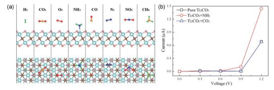
Fig. 6 (a) Schematic illustration of the adsorption of  $NH_3$ ,  $H_2$ ,  $CH_4$ , CO,  $CO_2$ ,  $N_2$ ,  $NO_2$  and  $O_2$  molecules on monolayer  $Ti_2CO_2$ . (b) Current–voltage relationship before and after the adsorption of  $NH_3$  or  $CO_2$  molecule on monolayer  $Ti_2CO_2$ . Reprinted from ref. 62 with permission. Copyright 2015 American Chemical Society.
