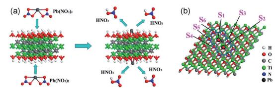
Fig. 3 (a) Schematic illustration of the formation of the  $Ti_3C_2(O_2H_{2-2m}Pb_m)$  structure from  $Ti_3C_2(O_1)_2$  to  $Ti_3C_2(O_2H_{2-2m}Pb_m)$ ; (b) top-view of the  $Ti_3C_2(O_2H_{2-2m}Pb_m)$  structure when the Pb coverage is 1/9 ML. S1–S6 represent the different atom sites of the hydroxyl. Reprinted from ref. 44 with permission. Copyright 2015 American Chemical Society.
