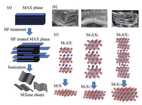
Fig. 1 (a) Early reported three different structures of MXenes (non-terminated):  $M_2X$ ,  $M_3X_2$  and  $M_4X_3$ . Reprinted from ref. 22 and 23 with permission. (b) SEM images of  $Ti_2AlC$ ,  $Ti_3AlC_2$  and  $Ta_4AlC_3$  after HF treatment (from right to left). (c) Schematic illustration of the synthesis of MXenes from MAX phases. Copyright 2013 John Wiley and Sons and Copyright 2012 American Chemical Society.
