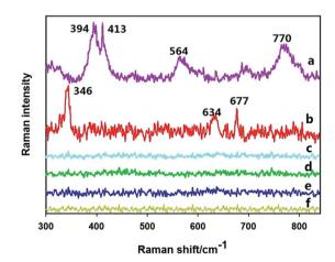
Fig. 2 SERS spectra of an apple surface containing (a) omethoate pesticide and gold nanoparticles, (b) chlorpyrifos pesticide and gold nanoparticles, (c) omethoate pesticide only (d) chlorpyrifos pesticide only, (e) gold nanoparticles only, (f) a clean apple surface.
