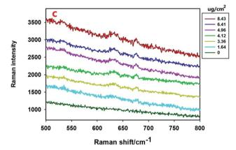
Fig. 3 Average SERS spectra of apple surfaces (a) with different omethoate contents, (b) with different chlorpyrifos contents. Average SERS spectra of leaf surfaces (c) with different chlorpyrifos contents.
