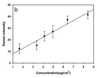
Fig. 4 (a) Regression curve of the Raman peak (at  $413~\rm cm^{-1}$ ) intensity and omethoate content on the apple surface. (b) Regression curve of the Raman peak (at  $346~\rm cm^{-1}$ ) intensity and chlorpyrifos content on the apple surface. The error bar indicates the standard deviation of the measurement.
