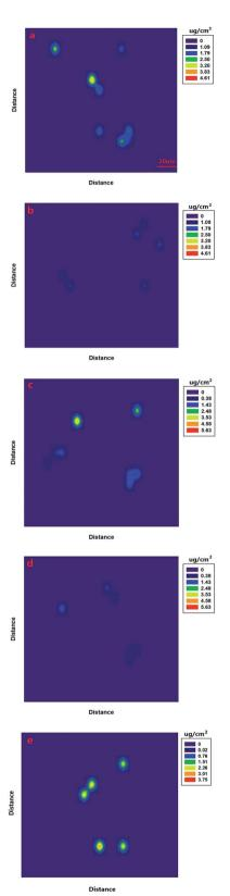
**Fig. 6** SERS imaging of the omethoate solution sprayed on the apple surface with concentration of (a) 0.201 g L $^{-1}$  and (b) 0.105 g L $^{-1}$ . SERS imaging of the chlorpyrifos solution sprayed on the apple surface with concentration of (c) 0.201 and (d) 0.105 g L $^{-1}$ . (e) SERS imaging of the chlorpyrifos solution sprayed on the leaf surface with concentration of 0.201 g L $^{-1}$ .
