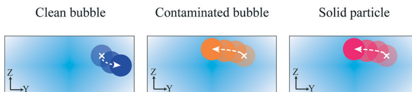
Fig. 13 Schematic of the equilibrium position of a bubble in a clean carrier fluid (left), a bubble in a carrier fluid with surfactants (middle), and a solid particle (right). Different circles show the position of circles at different times (x marks the initial position). The clean bubble goes to the center in the Z direction and moves towards the shallower wall. The solid particle and contaminated bubble move towards the center of the wider channel and stay centered in the Y direction.
